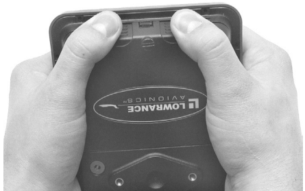
Replace battery compartment cover: Slide cover into place, left. Press in cover's bottom edge, right
